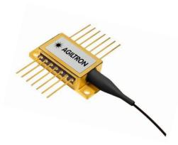
The 850nm series laser diodes are fabricated in a hermetically sealed 14-pin butterfly package. The laser diodes contain a monitor photodiode, thermoelectric cooler (TEC), and a thermistor to secure high-quality laser performance. Our laser products are Telcordia GR-468 qualified and in compliance with RoHS Directives.
